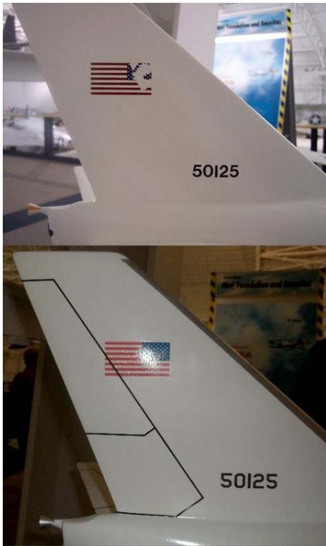
I made replacements for the missing wingtip and tail tip antennae from Evergreen tubing sanded to shape. Holes were pre-drilled for mounting with a brass tube into the wing and into the antenna. I waited for final assembly before mounting them. The whole model was transported back to the museum the following Saturday and assembled in the display location.
