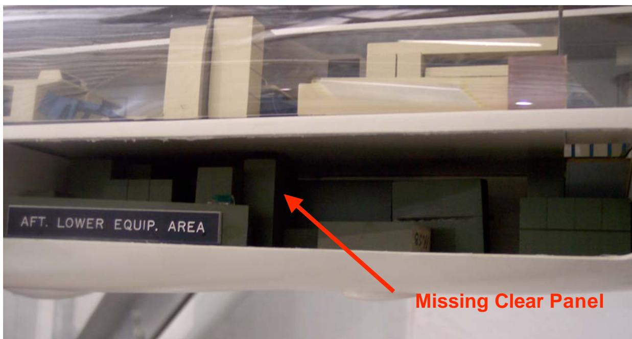
The toughest part of the project was the clear panel for the lower rear equipment bay that was missing. There are actually two clear panels for the lower bay, but the smaller one was found inside the model. I made a new master for the missing piece using PVC and Bondo. It turned out I have a vacuform platen big enough to do the piece, so I bought a sheet of clear from Hobbytown and manufactured the replacement part.
